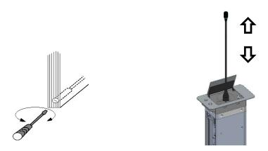
CONMIC FLAP is equipped with DIRECT AXLE ACCESS (DAA), a useful feature for installation and maintenance. This allows you to extend and retract the microphone manually, i.e. without a power supply. Access is located on the right and left bottom of the side of the case. You will need a slotted screwdriver or a cordless screwdriver to operate it.
